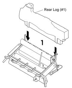
Figure 17 - Installing Rear Log
